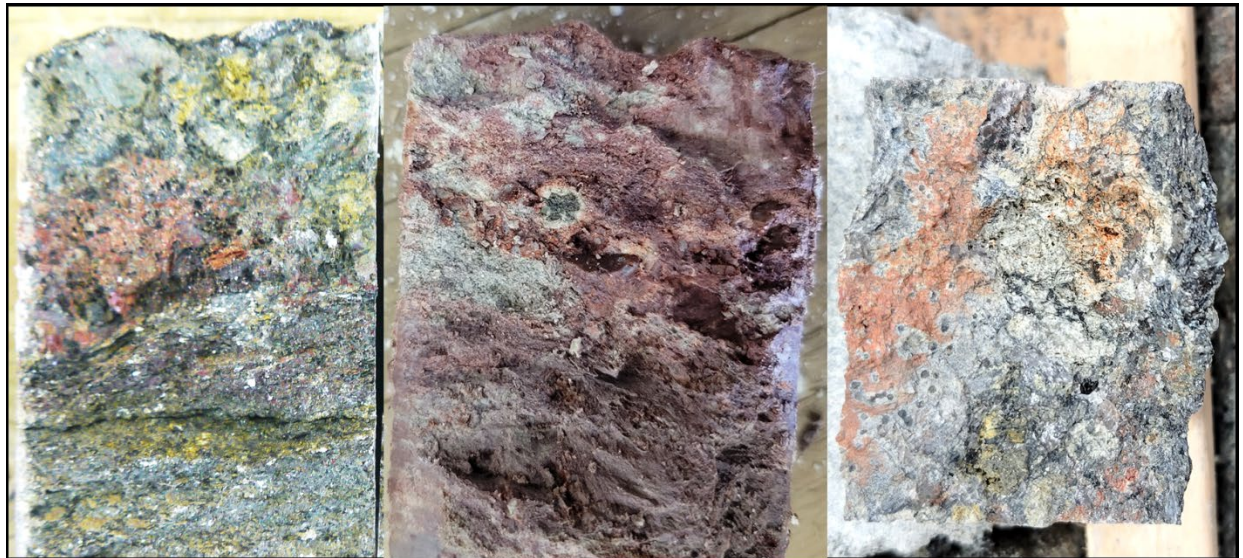
Figure 3: Uranium mineralization on core returned from WO-2 and WO-4. A total of 393 core samples have been sent to the Saskatchewan Research Council geochemical laboratories for analysis. Uranium can be seen as yellow oxides or as black spots with white reaction rims.
