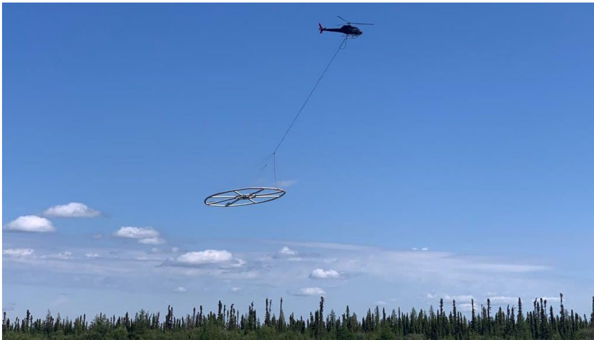
Figure 1: The Axiom Xcite TDEM airborne system in action.
