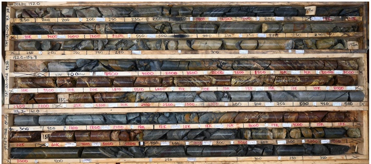
Figure 3 TAT23-002 drill core from the mineralized section (147.1 to 161.0 m). Scintillometer readings are written on the core boxes in counts per second and were measured using a digital, hand-held CT-007M scintillometer by Environmental Instruments Canada Inc.
