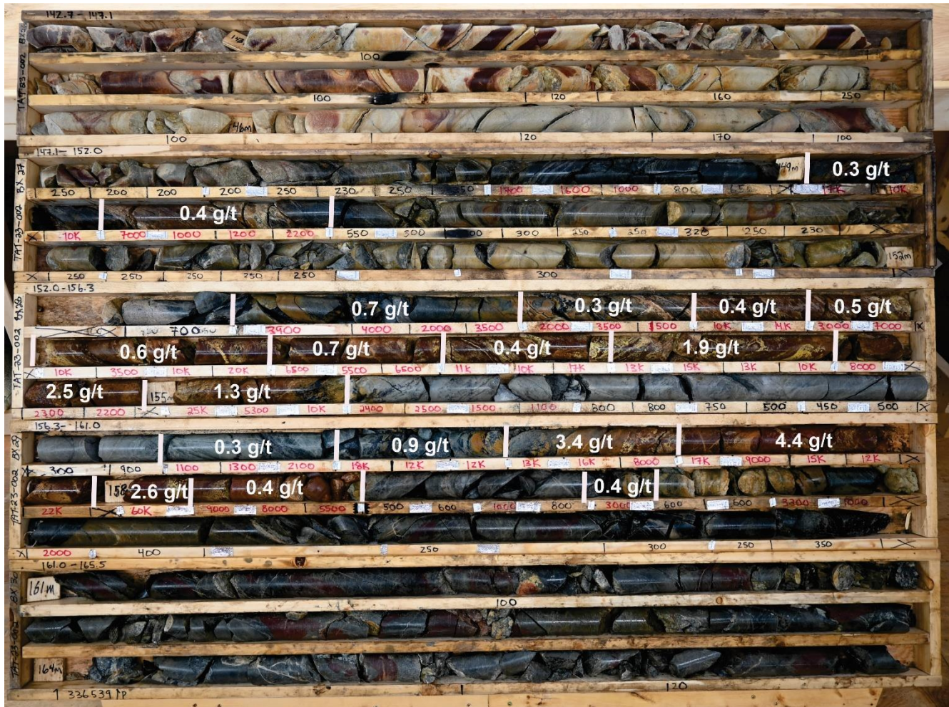
Figure 3 TAT23-002 drill core from the mineralized section (142.7 to 165.5 m). Scintillometer readings are written on the core boxes in counts per second and were measured using a digital, hand-held CT-007M scintillometer by Environmental Instruments Canada Inc. The fire assay Au values are shown within the U assay intervals.
