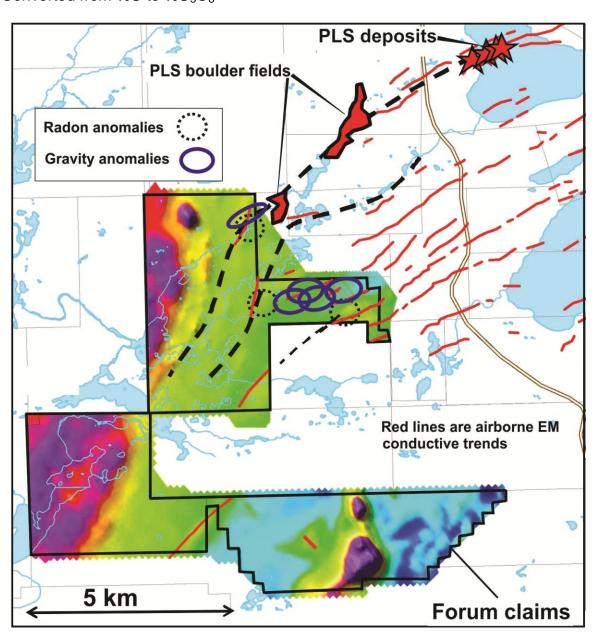
**Figure 1:** Gravity and radon anomalies with EM conductors on Forum's Clearwater Project. Red lines are airborne EM conductors, black dashed lines are interpreted structural trends. The background colours are from an airborne magnetometer survey. Forum plans to drill the gravity, radon and EM targets in February.
