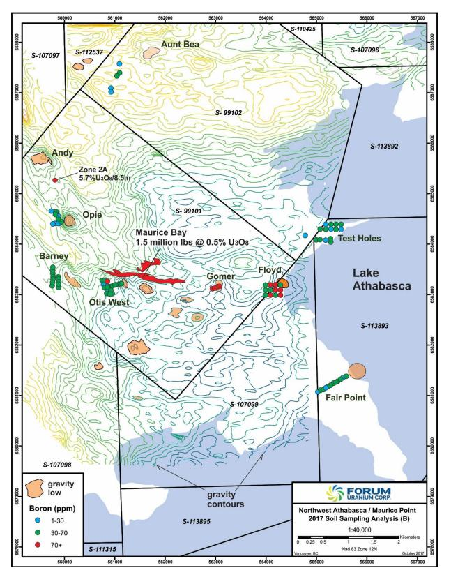
**Figure 1: Soil Sample Results on NWA/MP Projects**. The contours are the gravity survey with the orange fill being the anomalously low areas.
