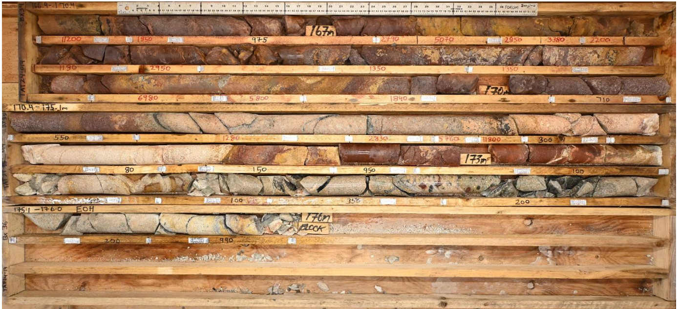
Figure 5 TAT24-014 drill core from the mineralized section at approximately 166.5 – 176.0 m. The uranium mineralization is largely hosted in steep brittle structures within a psammopelitic and granitic unit. Scintillometer readings are written on the core boxes in counts per second and were measured using a digital, hand-held CT-007M scintillometer by Environmental Instruments Canada Inc.
