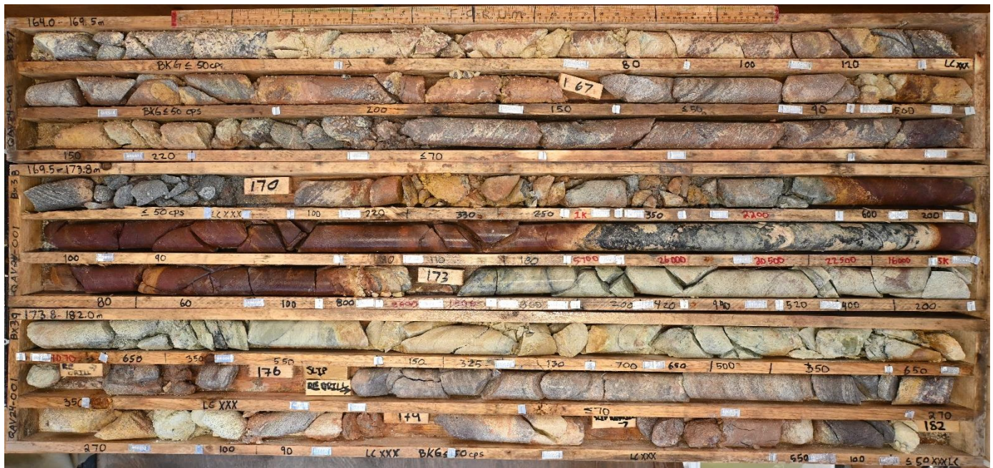
Figure 4 Core photo of the 0.5 m mineralized lense that intersected 8.2% U3O8 at 172.0 to 172.5 m.
